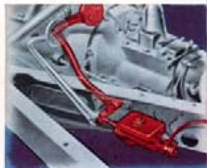
The master hydraulic cylinder is bolted to a rigid pedal bracket. A floor board inspection plate makes it easy to check the quantity of fluid.
